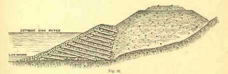
illustrates the manner in which crib-wharfing was constructed when the line encroached on the river. The embankment was faced with rip-rap, interlaced with a rough framework of cedar timbers, as a precaution to prevent inroads by flood-water on the newly formed earthwork.
